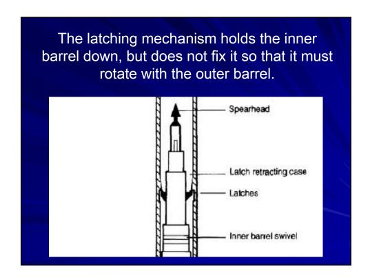
When the outer and inner barrels have been drilled for the length of the run, the wire line is winched upwards, and the latching mechanism automatically disengages the inner barrel from the outer. The inner barrel and core are hoisted to ground surface, where the core is extracted and a new length of outer barrel is added to the string.
