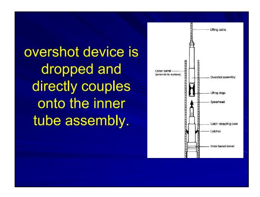
An overshot device is dropped on a cable and directly couples onto the inner tube assembly, allowing fast retrival of the core after each core run.
